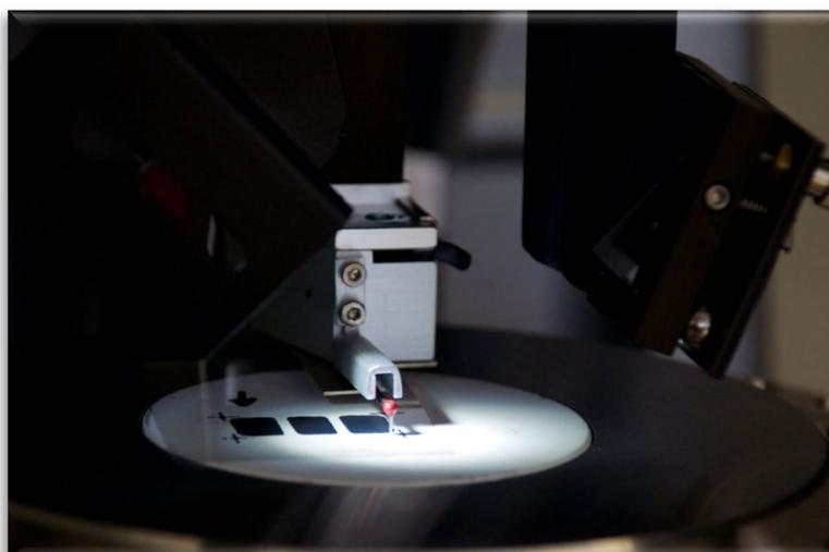
Figure 24 Close up of the cantilever probing a sample (source: ENAS)
