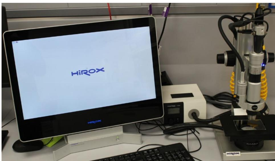
Figure 9 Optical microscope, Hiox KH-8700 (source: JMFC)
