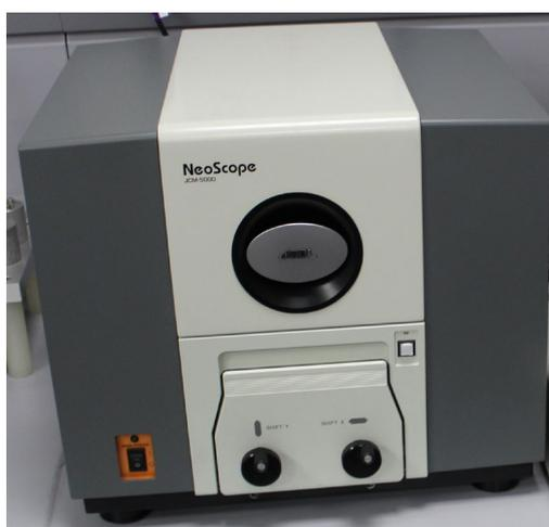
Figure 14 – JEOL NeoScope JCM 5000, Scanning Electron Microscope (source: JMFC)
